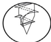
Specially formed tip for a clearly faster fixing of screws in comparison to most competitor's screws
