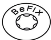
Torx screw head for better grip of the bit
